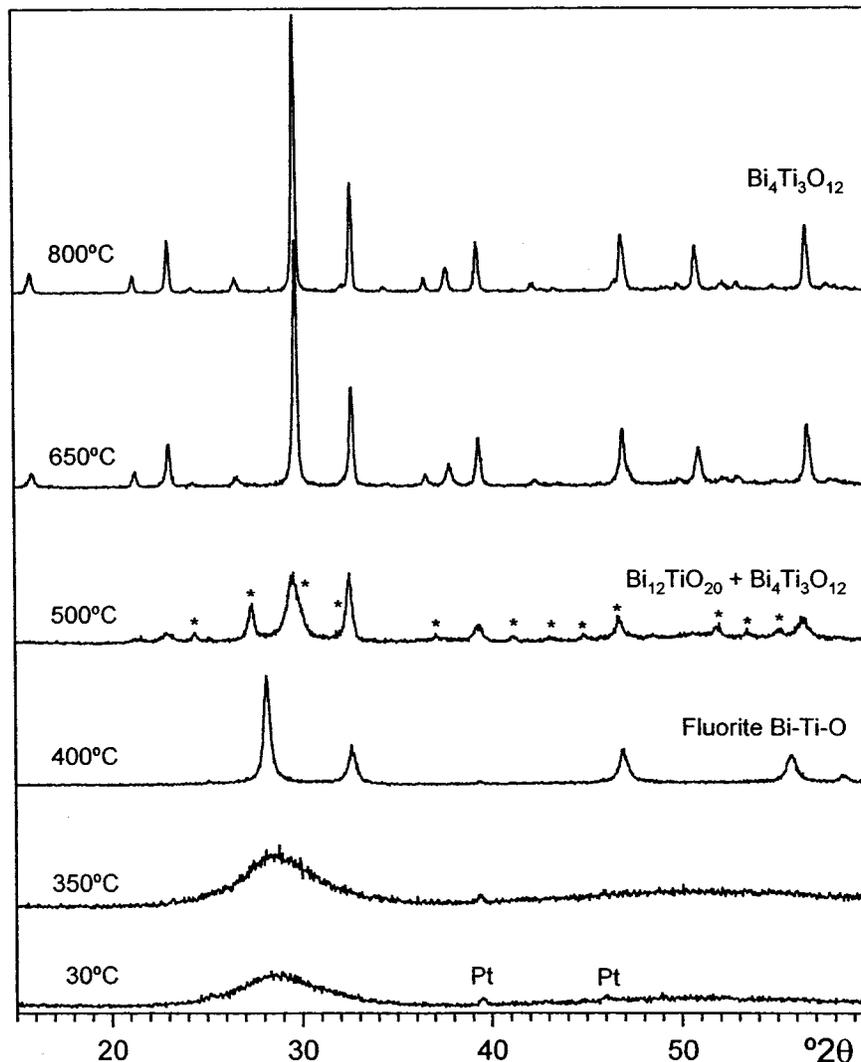
**Figure 4.** XRD recordings taken at increasing temperatures of the planetary milling precursor (19 h of mechanical grinding; \*,  $\text{Bi}_{12}\text{TiO}_{20}$ ).
