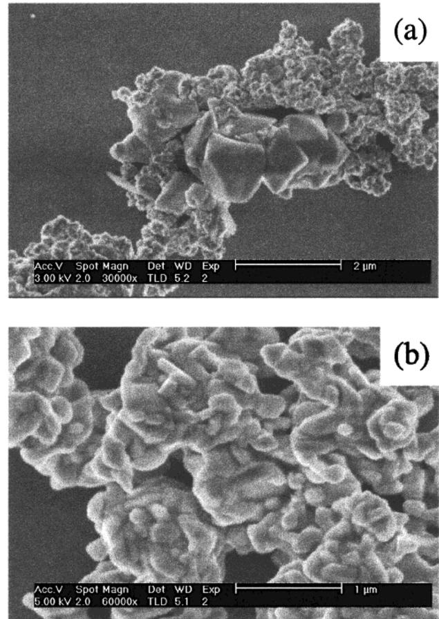
**Figure 6.** Scanning electron micrographs of the vibrating ball-milling precursor annealed at (a) 500 °C for 12 h (Bi–Ti–O fluorite) and (b) 600 °C for 3 h ( $\text{Bi}_4\text{Ti}_3\text{O}_{12}$  Aurivillius phase).
