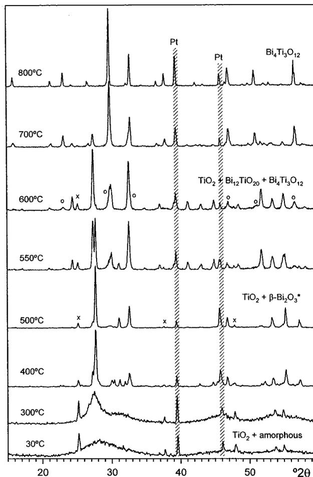
**Figure 3.** XRD high-temperature patterns recorded for the *n*-butylamine precursor ( $\times$ ,  $\text{TiO}_2$ ;  $\circ$ ,  $\text{Bi}_4\text{Ti}_3\text{O}_{12}$ ; dashed lines, Pt (sample holder); \*,  $\beta$ - $\text{Bi}_2\text{O}_3$  is partially doped).
