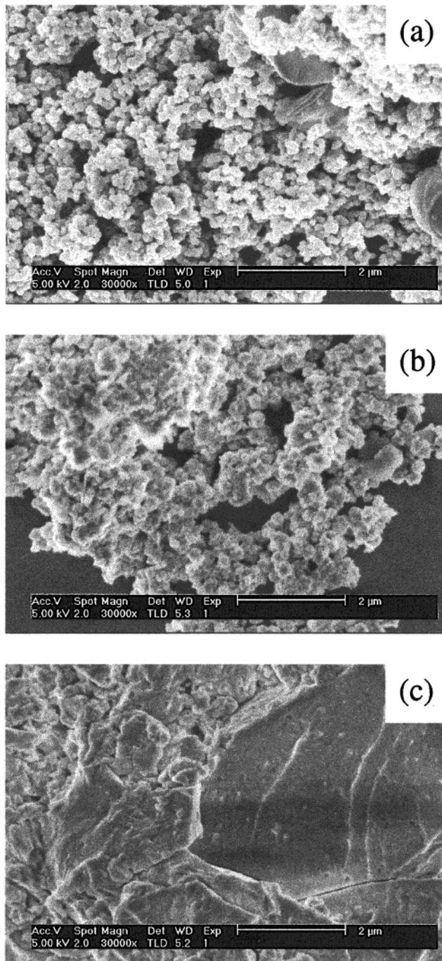
**Figure 5.** Scanning electron micrographs of (a) the initial  $4\text{Bi}_2\text{O}_3:3\text{TiO}_2$  oxide mixture, (b) vibrating ball milling (168 h), and (c) planetarium (72 h) amorphous precursors.
