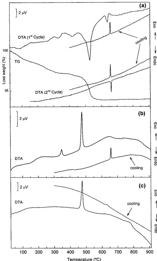
**Figure 2.** DTA curves of (a) the *n*-butylamine precursor and the amorphous ones obtained from (b) vibrating ball (168 h) and (c) planetary mills (72 h). TG curve and two cooling/heating cycles are also shown in (a).
