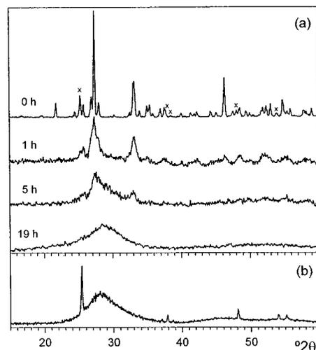
**Figure 1.** XRD recording taken at room temperature of (a)  $4\text{Bi}_2\text{O}_3:3\text{TiO}_2$  oxide mixture after different milling times. The grinding was carried out by a planetary mill; (b) precursor obtained in the *n*-butylamine method (x,  $\text{TiO}_2$  (anatase)).
