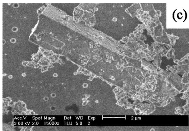
**Figure 8.** Scanning electron micrographs of (a) *n*-butylamine precursor and treated at (b) 520 °C for 1 h ( $\text{Bi}_{12}\text{Ti}_{20}$ ) and (c) 750 °C for 1 h ( $\text{Bi}_4\text{Ti}_3\text{O}_{12}$ ).
