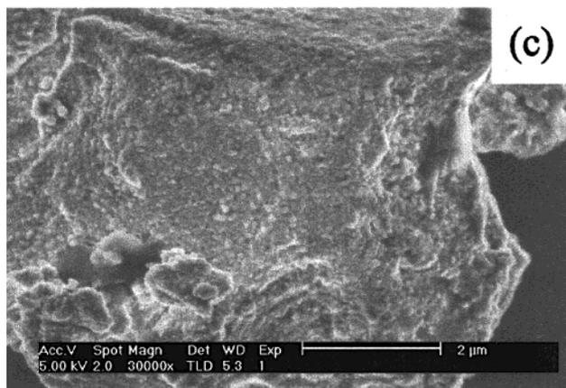
**Figure 7.** Scanning electron micrographs of (a) Bi-Ti-O fluorite obtained from the planetarium precursor (19 h) treated at 350 °C for 1 h. (b) and (c) correspond to  $\text{Bi}_4\text{Ti}_3\text{O}_{12}$  Aurivillius powders attained at 600 °C for 1 h. The precursors were mechanoactivated with the planetarium mill for 19 and 72 h, respectively.
